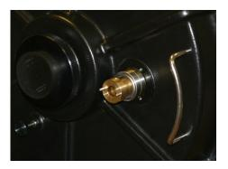
Slide the Ring Adapter over the brass focus shaft. The two pins should be pointing out away from the telescope. Lock in place using a 1/16" hex-head wrench to tighten the small set screw in the side. It will help in mounting the focuser to rotate the pins so they are aligned side-by-side. (Looking at the back of the telescope, the left pin should be aligned with the left mounting hole from where the original cover plate was removed.)
