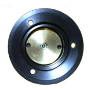
Hold the MicroFocuser with the "Feather Touch Focuser" logo on top. Look into the inside of the focuser at the brass plate with the two holes in it. Rotate the black focus knob until the holes are oriented side-by-side. (Looking into the focuser with the logo on top, the right hole in the brass plate should line up with the right mounting hole in the base of the focuser.)
