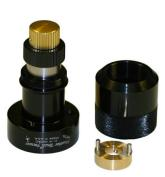
Begin by separating the 3 components of the SCT MicroFocuser. Remove the packing foam from the inside of the focuser. This will allow the Adapter Ring to drop out of the inside of the focuser. Remove the Knurled Sleeve from the main focuser. The Sleeve protects the focus knob during shipping and covers the mounting screws when the focuser is attached to the telescope.
