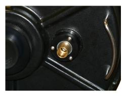
Telescopes with metal knobs are removed by loosening the small set screw in the side of the knob using a 1/16" hex-head wrench. Rubber focus knobs can just be pulled off. This will expose the brass focus shaft to which the MicroFocuser will be attached.
