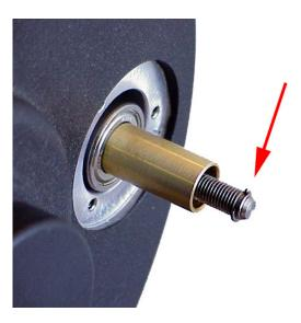
The C-clip at the end of the focus shaft must be removed to install the SCT Micro-Focuser. The clip should be removable by hand, but you may use needle-nose pliers or a similar tool if necessary. Be careful not to scar the threads of the focus shaft as the SCT Micro-Focuser must be threaded on in a later step. If your telescope has a screw, simply remove this with a screwdriver.
