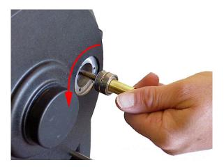
Rotate the brass portion of the focus shaft *counterclockwise*. This will unthread the brass shaft and bearing assembly from the threaded rod. Remove these parts entirely (you will turn the brass shaft quite a few times to remove it).
