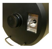
Turn the brass focus shaft counterclockwise to remove it from the threaded focus rod. This will take quite a few turns. Once the bearing assembly is removed, only the threaded focus rod (which pushes and pulls on the mirror cell to focus the telescope) will be left sticking out of the telescope as above.
