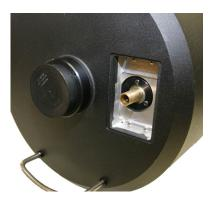
Remove the 4 screws holding on the rectangular outer cover plate. Keep these screws as they will be used later to attach the new MicroFocuser adapter plate.
