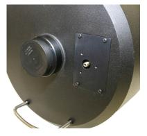
Use the original 4 screws to attach the included adapter plate. Be sure the beveled side is in toward the telescope. There is only one proper orientation for the plate, with the large hole on the left side.
