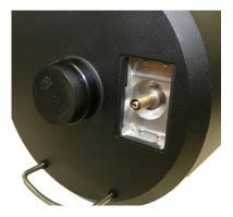
Use screwdriver to remove three screws from the focus assembly cover plate (the three screws around the outside of the focus shaft). Remove the cover plate. This can be tricky due to the plate being recessed. A knife blade or flat screwdriver can be helpful.
