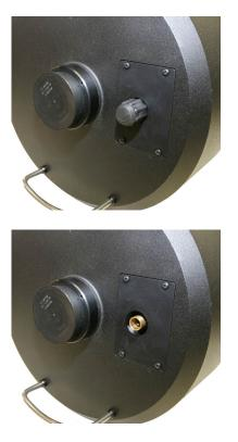
Begin by pulling off the rubber focus knob exposing the brass shaft underneath, as shown above.
