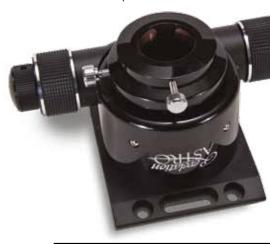
FINISHED IN GLOSS black, machined from a thick alloy and with generously sized controls, the 64mm-high Revelation Astro Newtonian Crayford Focuser Dual Speed has a bombproof feel. The thick-gauge drawtube has a 18mm-wide drive surface, which provides plenty of grip for the drive shaft, and the locking screw has a brass insert that fits in a deep milled slot.
