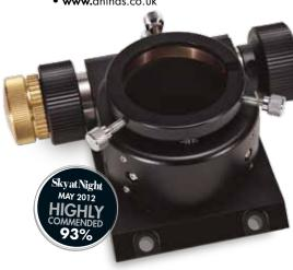
THE BAADER PLANETARIUM focuser exudes quality. Every feature is beautifully engineered, resulting in silky smooth operation. With a 44mm-high main body, this focuser has a low profile as well as a generous 30mm range of movement, although you may need a tube extension if you plan to use it for imaging.
