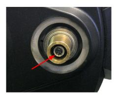
Rotate the brass portion of the focus assembly *clockwise*. This will bring the mirror back and expose the threaded portion of the focus shaft. At the tip of this threaded bolt will be a small Philips-head screw and washer. Remove this screw and washer, but keep them handy as they will be reinstalled later.
