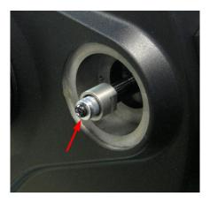
Thread the screw back into the end of the focus shaft.
