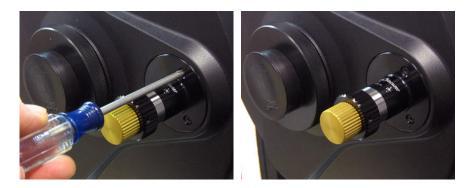
Use the three original screws to attach the SCT MicroFocuser to the telescope. You are now ready to head out under the stars! Use the black knob for coarse focus and the brass knob for fine focus (10:1 ratio). Note that the telescope will likely be pretty far out of focus, so you may need to turn the focus knob quite a few times to reach focus.
