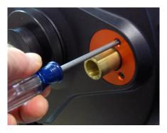
There are 3 small Phillips-head screws which hold the orange focus assembly cover in place. Remove these screws and take off the flat cover plate, exposing the inside of the focus assembly. These screws will later be used to attach the MicroFocuser.
