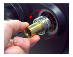
Rotate the brass portion of the focus shaft *counterclockwise*. This will unthread the brass cylinder and bearing assembly from the threaded rod. Remove these parts entirely (you will have to turn the brass shaft quite a few times to remove it).
