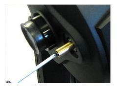
Rotate the brass portion of the focus assembly *clockwise*. This will bring the mirror back and expose the threaded portion of the focus shaft. At the tip of this threaded bolt will be a small Philips-head screw. Remove this screw, but keep it handy as it will be reinstalled later.
