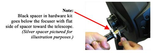
Thread the MicroFocuser into the brass stop. Hold the stop with a wrench and the black focus knob with the other hand to tighten the stop. *This stop MUST be tight to secure the MicroFocuser to the focus shaft.*
