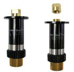
Unthread the stop from the end of the MicroFocuser. This stop prevents the telescope mirror from falling off the baffle tube inside the telescope. Thread the stop onto the focus shaft of the telescope. Be sure to thread the stop on far enough that the end of the threaded rod is exposed.
