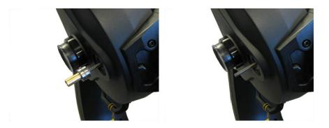
Rotate the brass portion of the focus shaft *counterclockwise*. This will unthread the brass cylinder and bearing assembly from the threaded rod. Remove these parts entirely (you will have to turn the brass shaft quite a few times to remove it).
