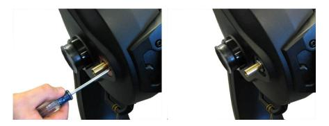
There are 3 small Phillips-head screws which hold the orange focus assembly cover in place. Remove these screws and take off the flat cover plate, exposing the inside of the focus assembly.
