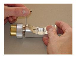
**2.a.** Remove the Feather Touch Micro from the shipping box and loosen the set screw to allow removal of the reduction assembly. Use the 1/16 Allen wrench that is supplied.
