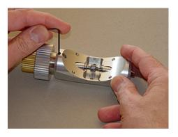
2.d. Fasten the reduction assembly to the pinion housing using the Allen wrench as shown. Do not over tighten, as this could damage the assembly. FINGER TIGHT IS ADEQUATE.
