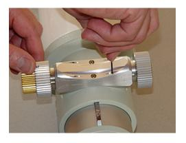
3.c. Insert the 1/16 Allen wrench into the adjustment hole and tighten leveling screws on the front side until you can see that contact is made between the leveling screw and the focuser housing. Do this for both sides. Then work on the back screws repeating the same steps.
