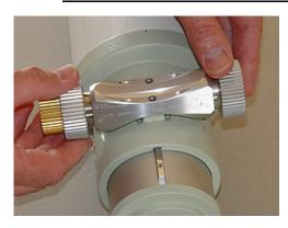
**3.a.** Place the pinion assembly on the Takahashi focuser housing as shown. The holes in the pinion housing should line up with the holes on the focuser housing. If they do not you may have to re-center the pinion.
