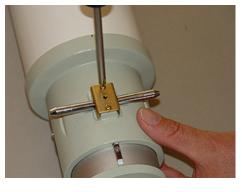
**1.e.** Remove the two Phillips screws that holds the pinion saddle in place.
