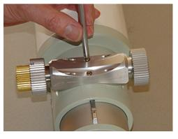
**3.b.** After placing the Phillips screws into the housing use the Phillips screw driver and drive the screws until they almost tighten the pinion housing. This step is important because you need to adjust the rack to the pinion by using these two screws and the four leveling screws with the 1/16 Allen wrench shown in the illustrations below.
