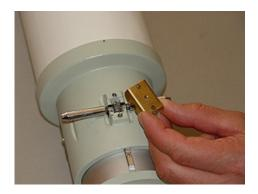
1.f. Remove the pinion saddle.
