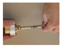
**2.b.** Take the Takahashi pinion and insert it into the reduction assembly as shown. If it is difficult to insert use the Allen wrench and loosen the screw on the locking collar.
