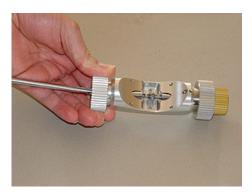
2.e. Insert the course focuser knob on the pinion and fasten it with the Phillips screw that is supplied. Hold the knob firmly while tightening the screw. Use a good Phillips screw driver so that the knob can be properly tightened and be careful not to slip.
