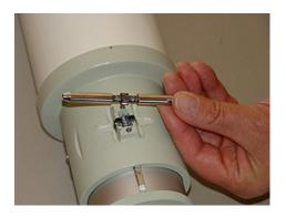
**1.g.** Remove the pinion from the focuser housing and place it on a clean piece of paper or paper towel.
