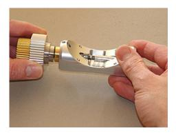
**2.c.** Insert the assembly into the pinion block as shown. If the pinion is too loose and moves during assembly, tighten the collar slightly using the Allen wrench. <u>Do not over tighten</u>. It will still need to be moved by hand during the adjustment phase.
