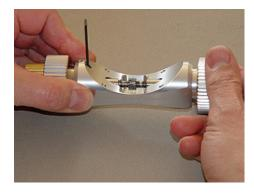
2.f. Rotate the pinion until the set screw is visible through the access hole and insert the 1/16 Allen wrench into the set screw. Holding the pinion assembly in one hand, twist the course knob slightly thereby moving the pinion relative to the pinion housing, and center the pinion relative to the cut out in the pinion housing. Firmly tighten the collar with the short lever being careful not to over tighten.
