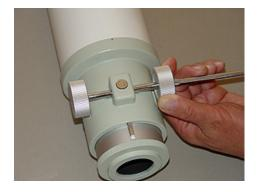
**1.b.** Remove the two focuser knobs using a standard Phillips screw driver as shown. Be careful not to slip.
