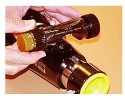
**2.c.** Place the Feather Touch Micro Pinion Assembly onto the TV focuser housing and move it back and forth slightly until you can feel the pinion and the screws nest into position.
