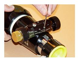
**2.d.** Using the Allen wrench, screw the (4) screws until they start to snug the Pinion Assembly to the focuser housing. This step is important because you need to adjust the rack and pinion by using these (4) screws and the (4) leveling screws with the 1/16 Allen wrench as shown in the next step.
