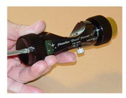
**2.a.** Remove the Feather Touch TVRF from the shipping box. Insert the coarse focuser knob on the pinion and fasten it with the Phillips screw that is supplied. Hold the knob firmly while tightening the screw. Use a good Phillips screw driver so that the knob can be properly tightened. <u>Be careful not to slip.</u>
