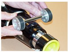
**1.d.** Remove the pinion assembly.
