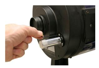
Use the 5/64" hex-head wrench to remove the three set screws holding the focus assembly in place.
