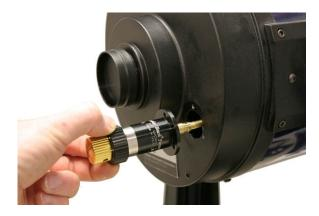
Tilt the outer portion of the MicroFocuser to the left as you did with the original focus assembly. Slide the inside tip of the brass shaft over the right end of the small rod on the mirror assembly.
