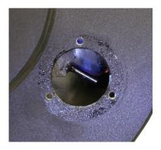
**Important:** The focus assembly (and the new Feathertouch SCT MicroFocuser) attaches to the internal mirror assembly via a small horizontal rod. This rod points outward away from the center of the telescope tube toward the right side (when looking at the back of the scope). You must slide the focus assembly off of this rod to remove the assembly.
