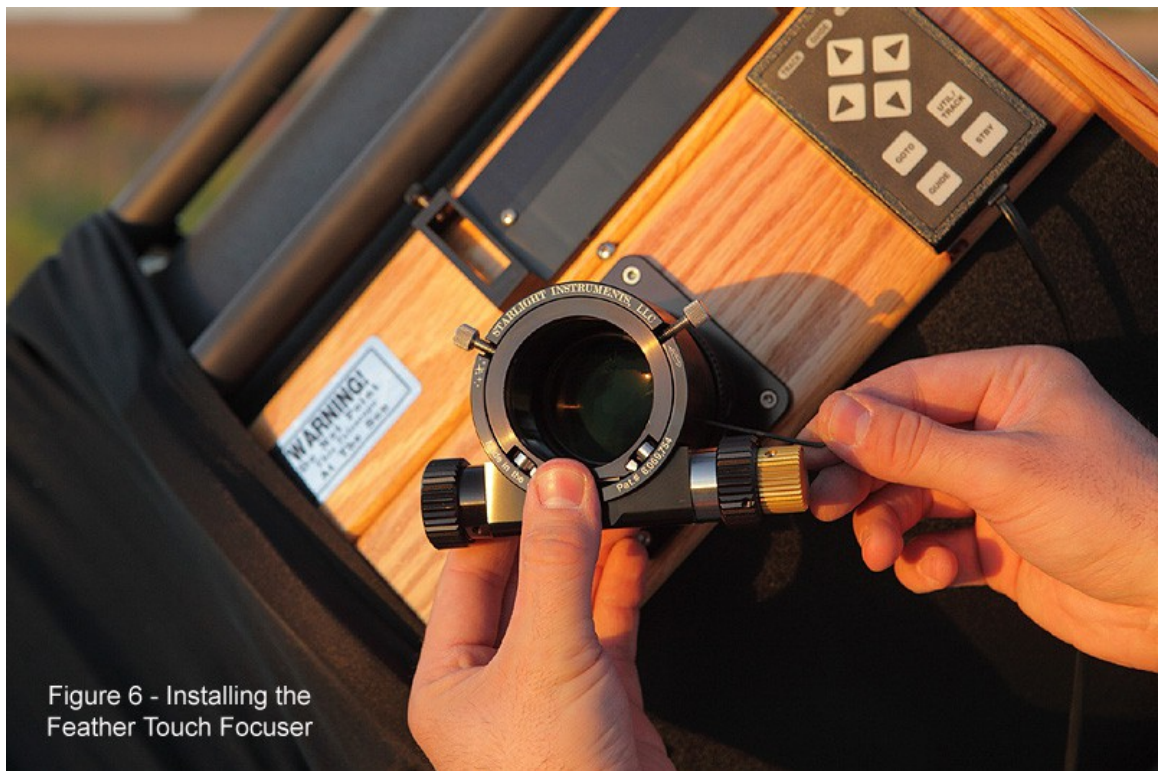
Figure 5 - Installing the Feather Touch focuser
