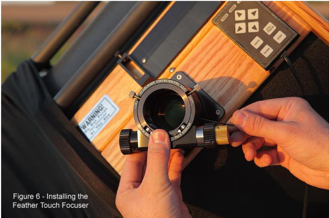
Figure 6 - Installing the Feather Touch Focuser
