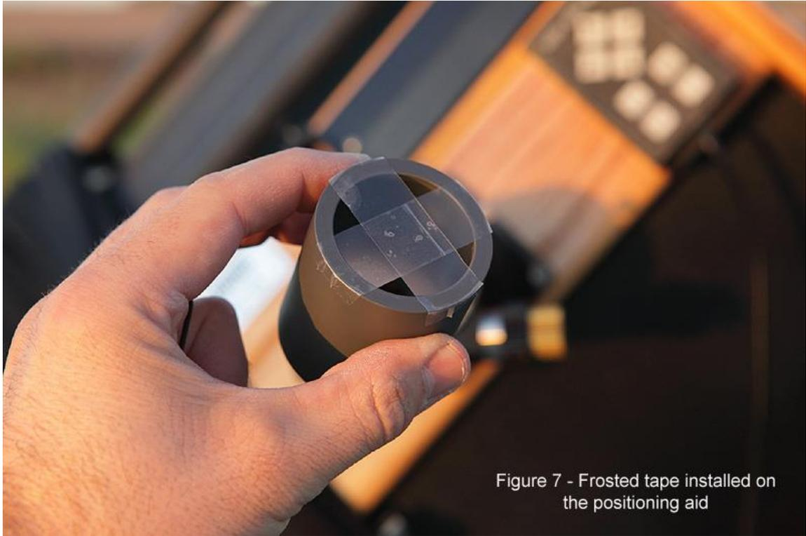
Figure 7 - Frosted tape installed on the positioning aid
