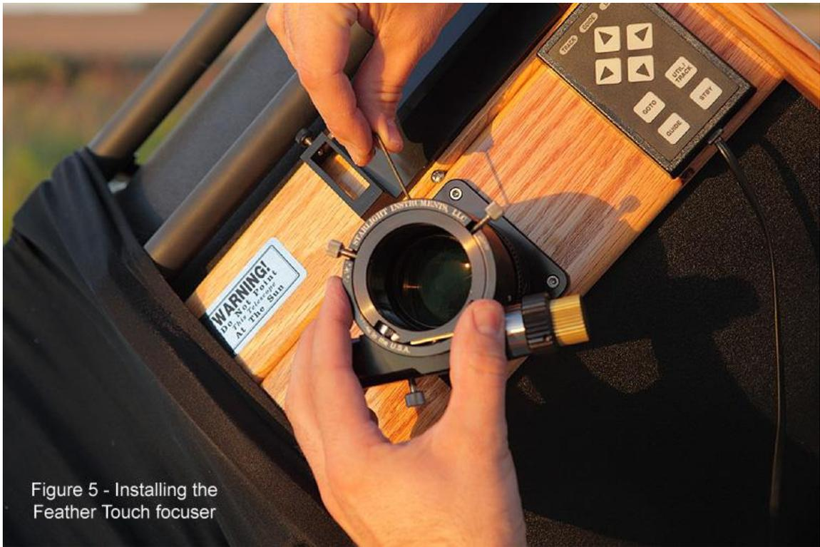
Figure 5 - Installing the Feather Touch focuser
