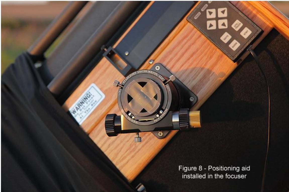
Figure 8 - Positioning aid installed in the focuser
