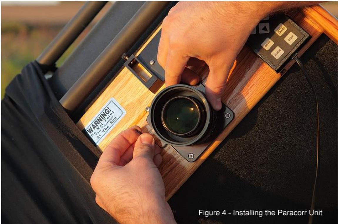
Figure 4 - Installing the Paracorr Unit
