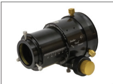
The 2.5" and 3.0" Feather Touch Focuser has a lifting capacity of 13-15 pounds and comes in draw tube travels of 1.5", 2.5", and 3.5".
