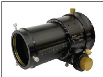
The True 3" Feather Touch Focuser will accept a 3" accessory and has a lifting capacity of 13-15 pounds and comes in draw tube travels of 1.5" and 3.5".
