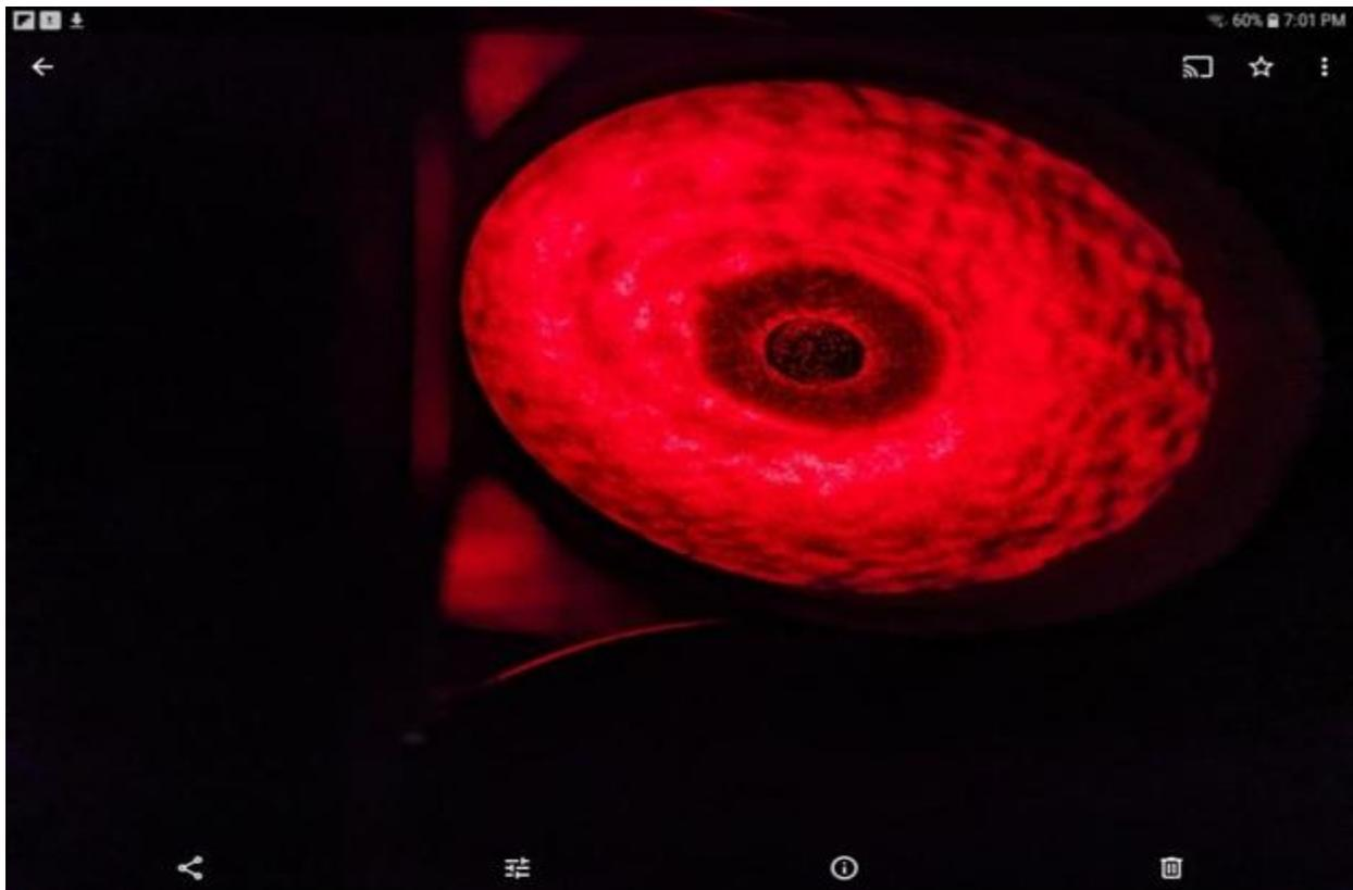
\*\*If the center marker is of a certain size, there will be a small red circle of light outside the central hole of the TuBlug screen and inside the shadow of the primary's center marker. You can use this as an aid to collimation by making that small illuminated ring perfectly uniform in thickness.
