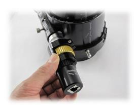
First start small pin into the gold knob and then slide clamp onto silver housing, this will most likely be a snug fit using a gentle back and forth motion slide the assembly together.
