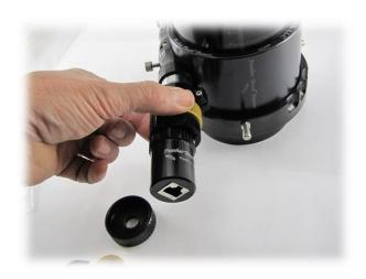
By turning the round motor housing counterclockwise you will disengage the gears, allowing manual use of the focuser, turn the motor housing clockwise to engage the gear for motor focusing.
