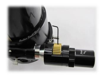
Make sure the gold knob is centered in the slot then tighten the gold knob using the 1/16 Allen wrench
