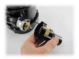
Put motor assembly onto pinion assembly
