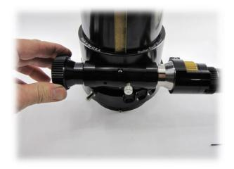
Turn black focus knob to make sure gold knob will not rub on motor housing If gold knob rubs and you can't fix it by adjusting the gold knob you can loosen the clamp assembly and move the entire assembly slightly in or out, the gold knob will remain tight to the small shaft.
