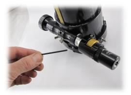
Using the 7/64 Allen wrench tighten the clamping screw
