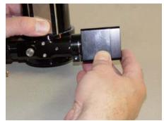
**1.f.** Slide the motor unit onto the Planetary Bell. Turn slightly if necessary to engage the gears.
