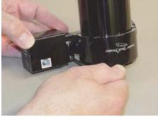
**1.g.** Fasten the Motor Unit by tightening the clamp collar using a 7/64 Allen wrench.
