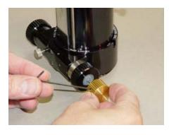
**1.a.** Place the focuser on a paper or a clean work surface as shown and remove the Fine Focus Knob with a 1/16 inch Allen wrench.
