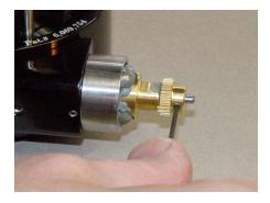
1.e. Attach the gear as shown with the hub towards the outside.
