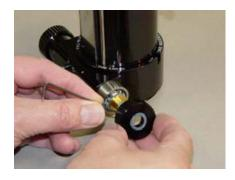
**1.b.** Remove the Course Focus Knob as shown with a 1/16 inch Allen wrench.
