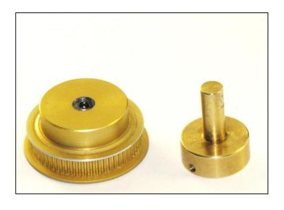
Remove shaft extension from pulley
