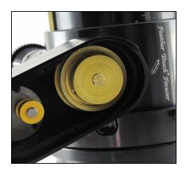
Make sure set screws are positioned over flats on shaft extension
