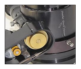
Utilizing the access hole tighten both of the pulley set screws
