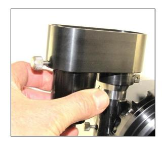
After timing belt is on both pulleys rotate motor housing clock wise to tension the belt
