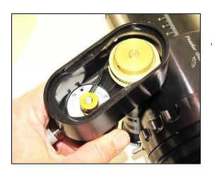
When the timing belt is tensioned tighten the thumb screw
